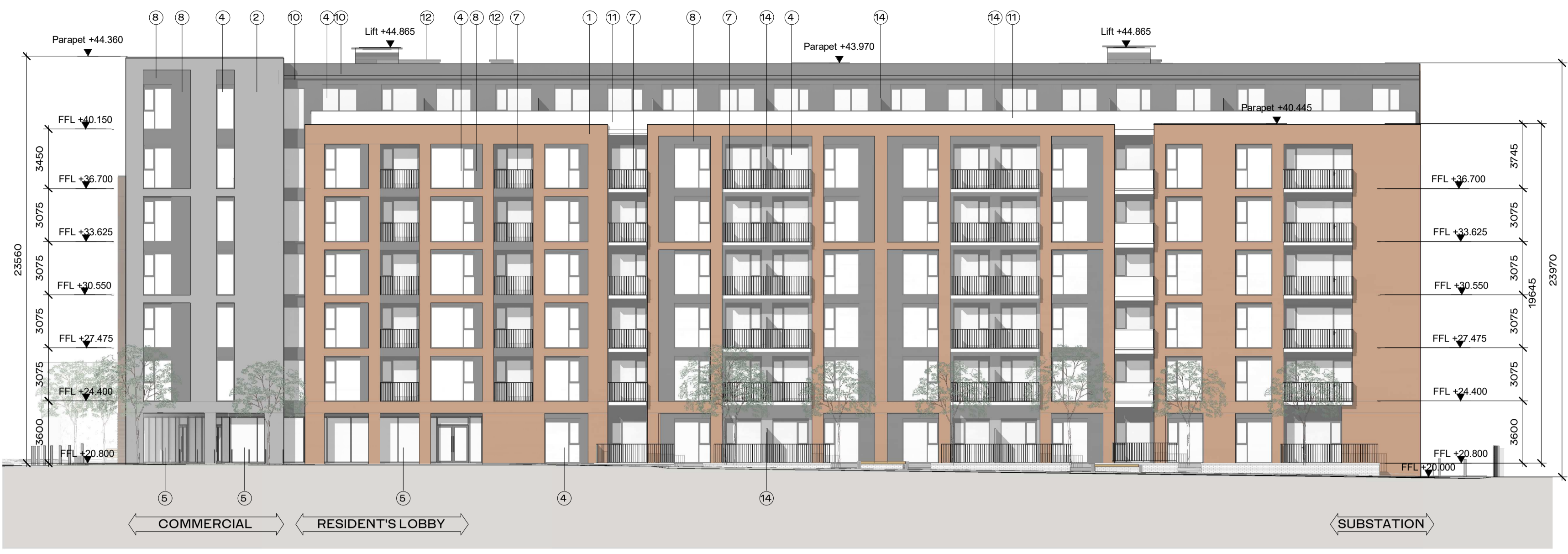
1 Block Elevation BG1 01 East Elevation 1 : 200
